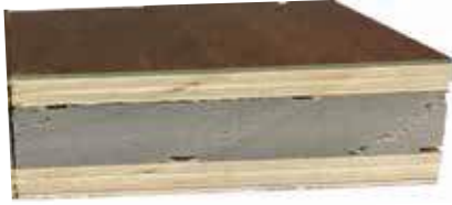
Presim special Thermik 38mm Betoform 8mm + EXPS 18mm + Betoform 8mm
